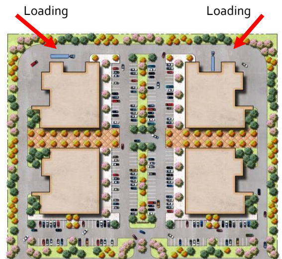
Figure 4. Appropriate location of loading areas.
