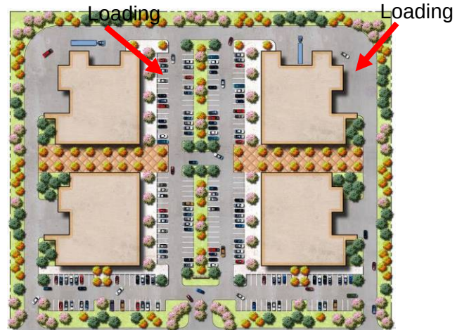
Figure 73. Appropriate location of loading areas.
